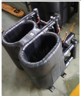
2. 304 stainless steel body, anti-corrosion ability is stronger, placed in the sea strong corrosive places can be long life 3. use 304 shell titanium tube The highest water temperature can reach 60 degrees
